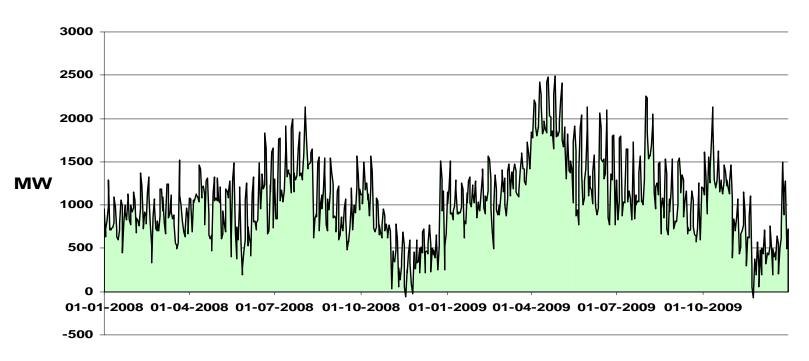
The Daily Peak Demand and Available Supply shown above is a companion graph shown with the Supply Cushion Metric as it provides a view of all capacity including wind and backup generation which are not in the Supply Cushion calculation. The companion graph enables participants to visually add or subtract supply or outage components to reflect their own supply assessments.
